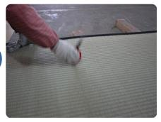
Checkers will carefully measure length, width and thickness of each tatami and deal with the mat, border and bottom.
