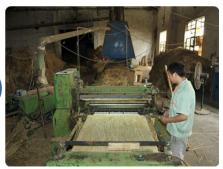
This machine will compress 7 layers rice straw into the demanded thickness, then cut into the specified length.
