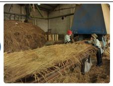
Plastic paper or igusa mat is on the bottom, put 2 layers rice straw. A machine will put 1 layer chopped rice straw, later put another 4 layers rice straw. So 7 layers of each tatami mat.
