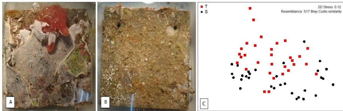
Figure 4: Typical recruitment of benthic organisms onto innovative concrete matrices (example from M4, 6 m post deployment, Red Sea). A) Textured face fully with 100% cover. B) Smooth face of the same tile with limited recruitment. C) 2D-MDS of community data. Each point represents one tile face (Textured face = Red square, Smooth face = Black circle). Example from Red Sea data, 6 m post deployment showing separation between textured (up) and smooth (down) tile face.
