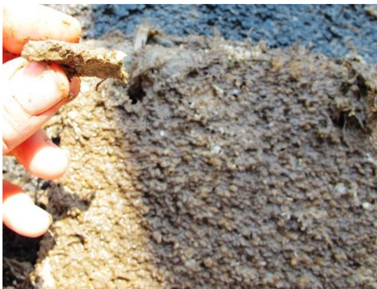
Figure 9: Scrapped material composed of calcitic biogenic growth accumulated onto an M4 tile 3 month post deployment.
